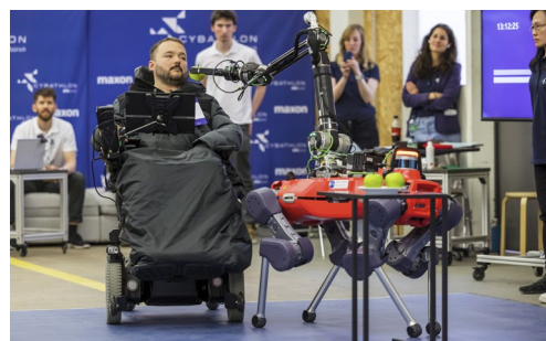
Envisioned approach 2: A person in a powered wheelchair and a robotic manipulator mounted to an auxiliary mobile platform.
