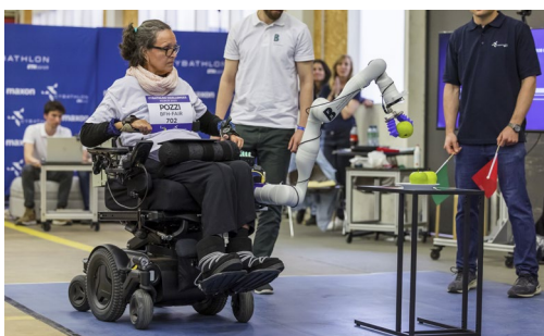
Envisioned approach 1: A robotic manipulator mounted to a powered wheelchair.
